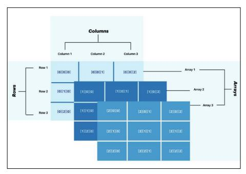
A 3-dimensional array is also allocated contiguous memory and is represented in memory, as shown below.
